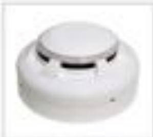
EVC-PY-IS Intrinsicly Safe Optical Detector For use in hazardous areas, good response to slowly developing fires. Y type chamber, good response to black smoke. Part No: 100-8300
